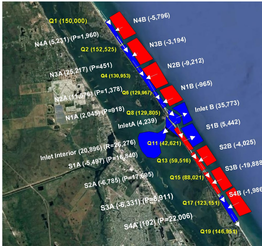
Figure 26. Annualized 17-year sediment budget for the summer 2007 to summer 2024. Values on the west of the barrier island indicate sand volume changes and values on the east indicate calculated sand flux rate in cubic yards per year. P= annualized placement quantities and R = annualized value of sand removed from the sand trap. Blue cells indicate sand volume increase whereas red cells indicate sand volume loss.
