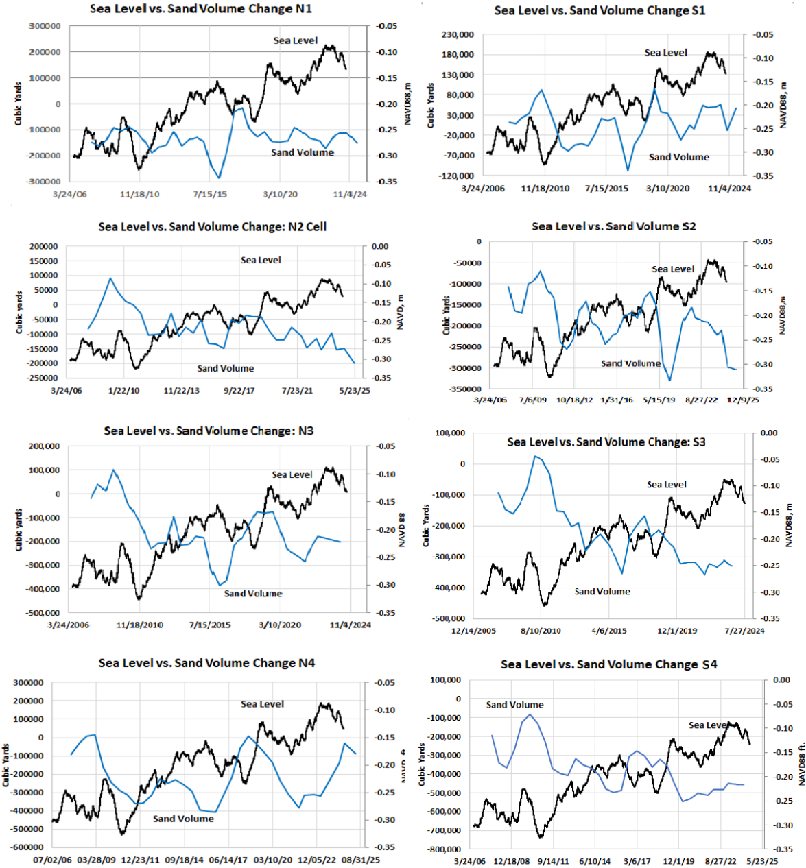
Figure 23. Comparison of sea level changes, cumulative sand volume changes within the sand budget cells to the north and south of Sebastian Inlet
