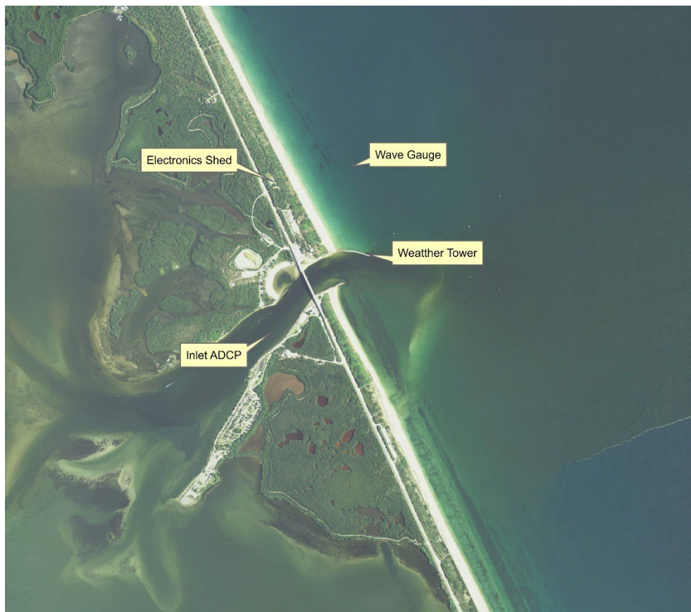
Figure 1. Location of Sebastian Inlet State Park oceanographic and meteorological instrumentation sites. The aerial photo and bottom topography are courtesy of the Sebastian Inlet District.
